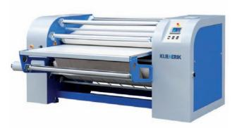
automatically transported (or 'flow') to the back of the calender in the exact same order. The transferred pieces of fabric can easily be gathered and sorted by size and colour or design. It is also possible to have the transferred pieces flow to the front of the machine by simply changing the directional plate under the infeed table. This feature is great for sampling or short runs.
