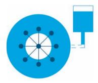
Klieverik heated drum: a unique concept. Completely filled with oil because of expansion vessel. Directly heated because heating elements are directly in the oil. Best temperature consistency due to thorough mixing of the oil.
